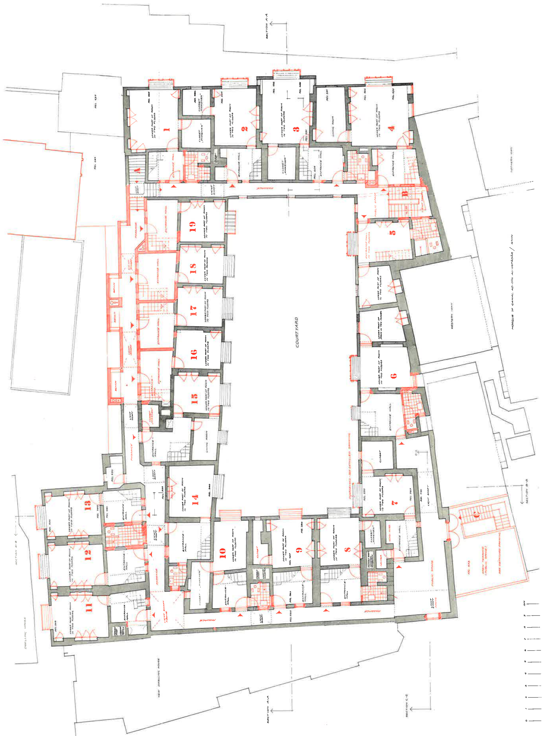
Abb. 53 Wakalat Bazar'a, plan of second floor, proposal for restoration; scale 1:200 (Flemming Aalund)
