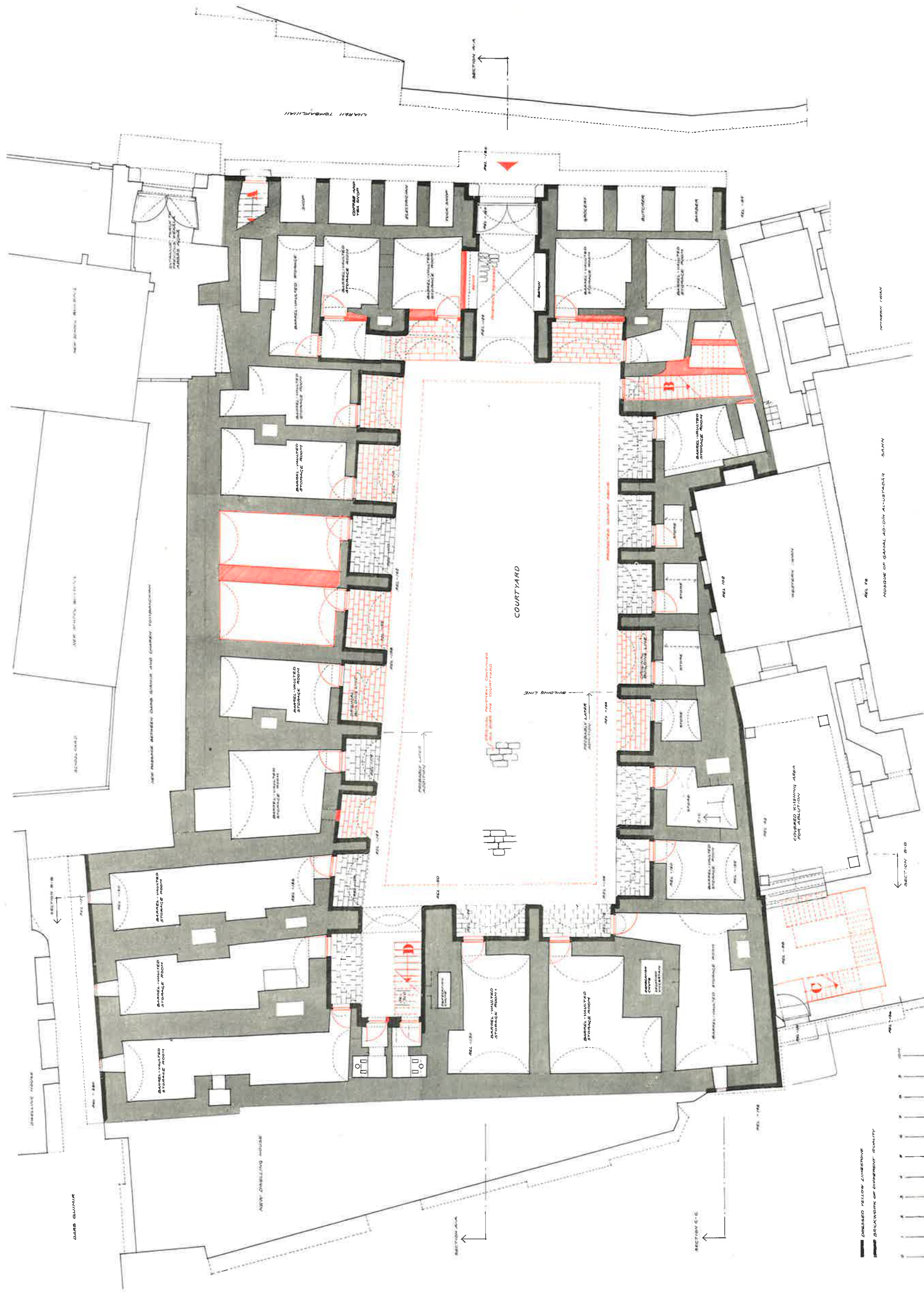
Abb. 49 Wakalat Bazar'a, plan of ground floor, proposal for restoration; scale 1:200 (Flemming Aalund)
