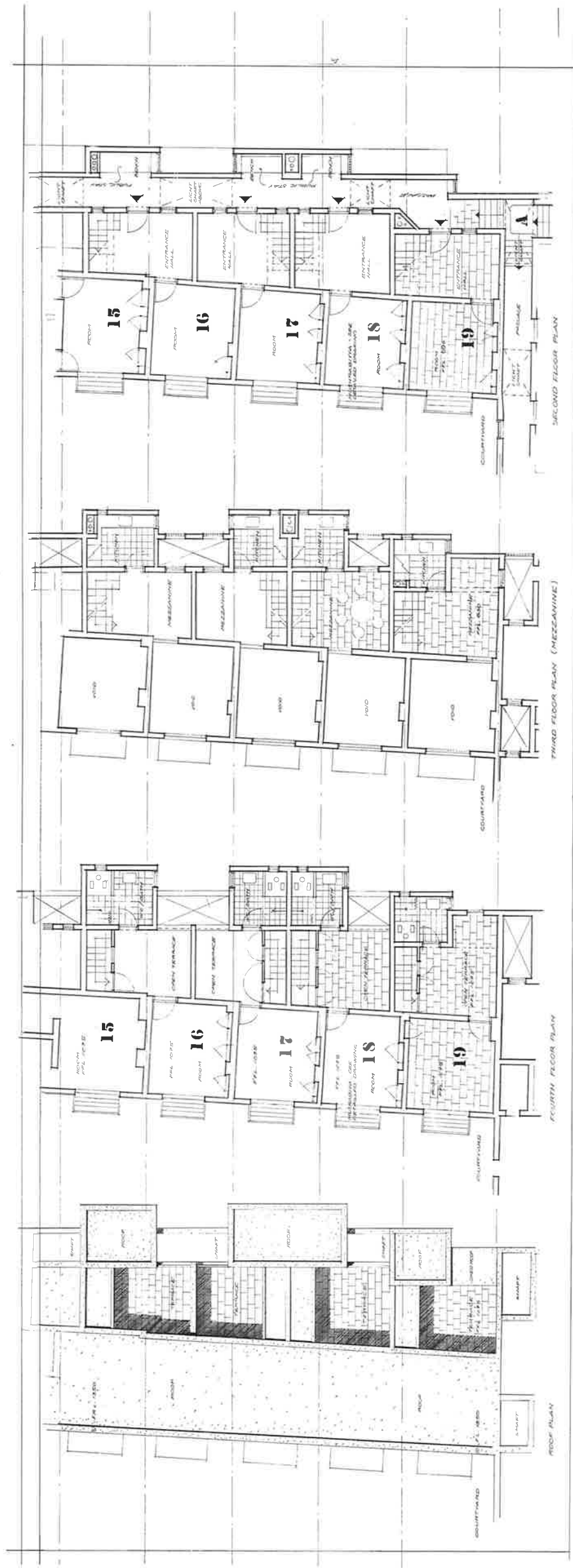
Abb. 59 Wakālat Bāzar'a, plans of flats nos. 15–19 in four levels, proposal for restoration; scale 1 : 200 (Flemming Aalund)
