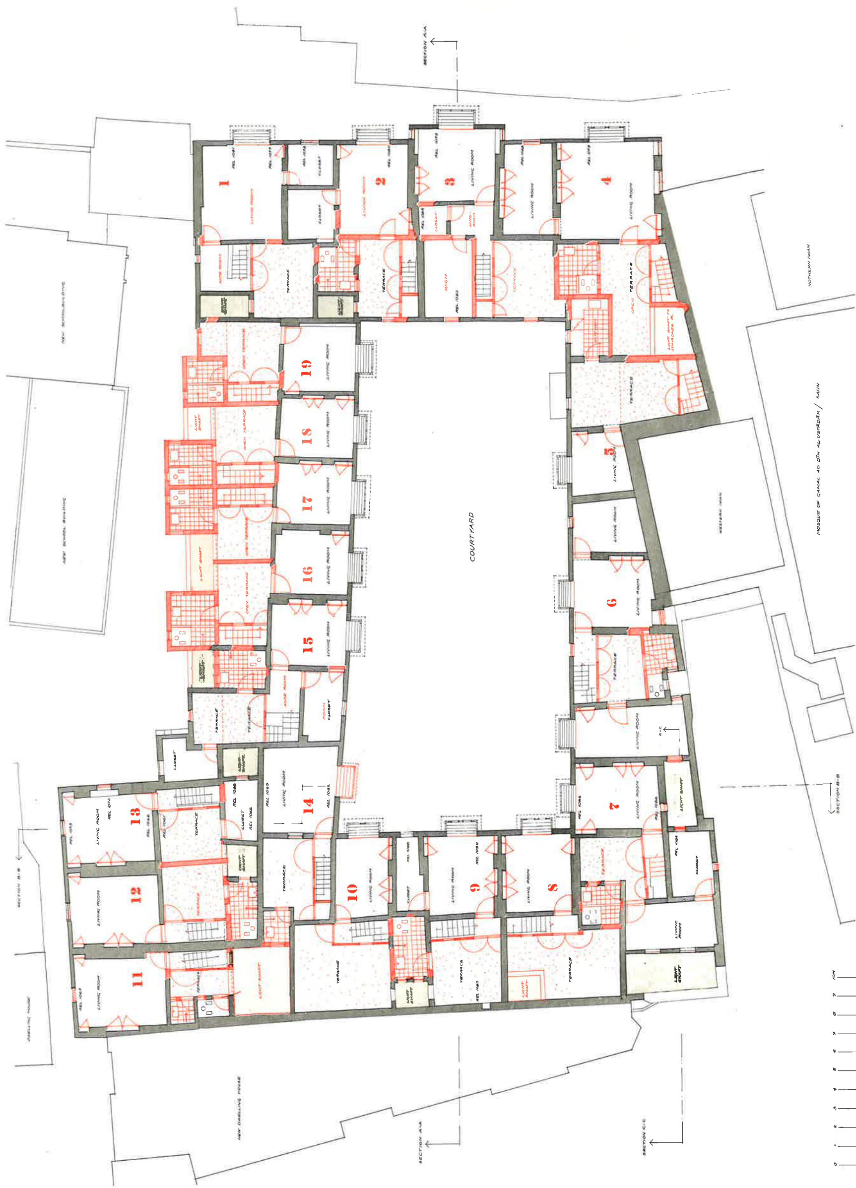
Abb. 57 Wakalat Bazar'a, plan of fourth floor, proposal for restoration; scale 1:200 (Flemming Aalund)
