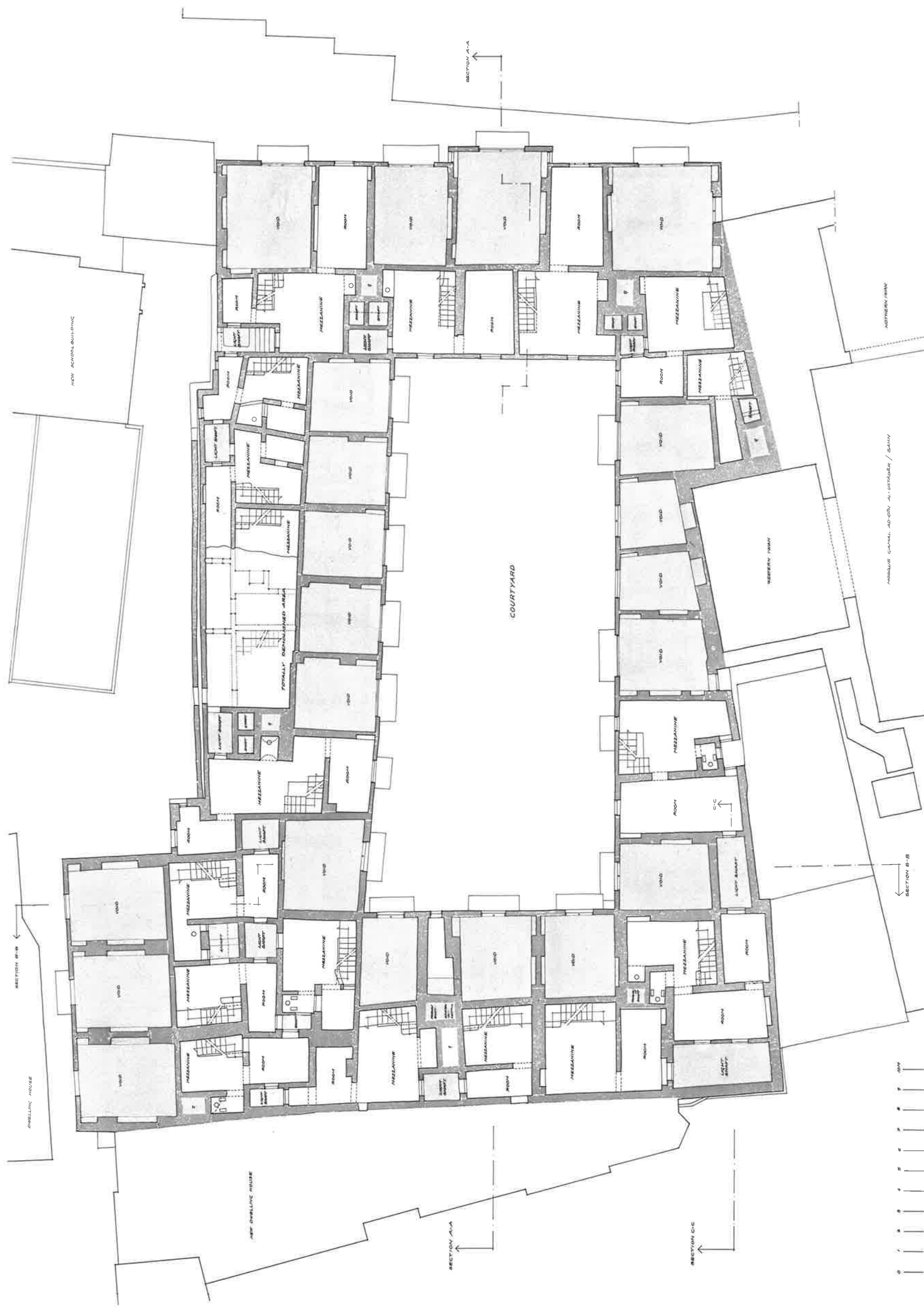
Abb. 54 Wakalat Bazar'a, plan of third floor (mezzanine), proposal for restoration; scale 1 : 200 (Flemming Aalund)
